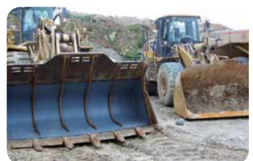
MATROX LINERS TO REDUCE HANG UP
