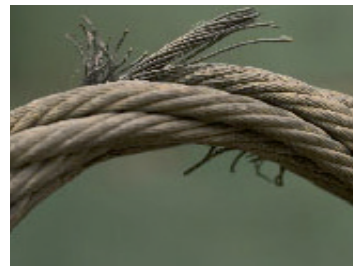
Figure 1. Strand break on six (6) lay wire rope.
